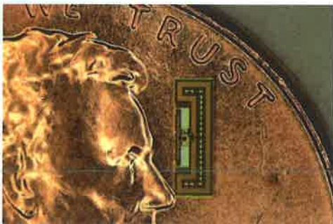
One example: An ant-sized radio on chip recently developed by Stanford and UC Berkeley
