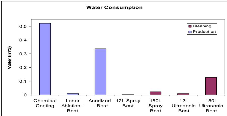
Figure 7 – Water needed to produce 1 m<sup>2</sup> self-cleaning and clean 1 m<sup>2</sup> surface [17]
