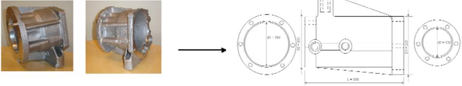
Figure 2: Automotive Transfer Case Picture and Drawing
