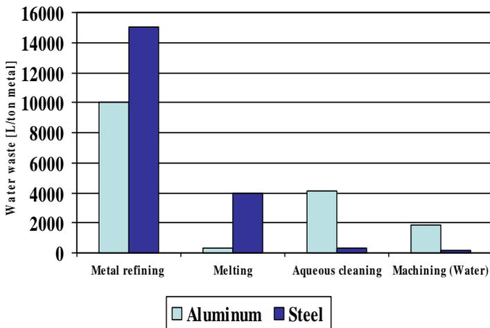
Figure 5: Water Consumption in Life-Cycle Processes [liters/ton] [7]
