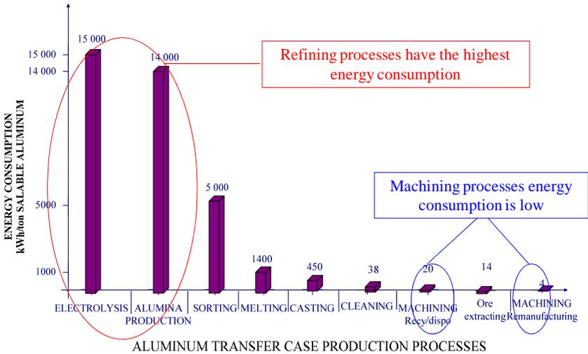
Figure 3: Transfer Case Energy Consumption [kWh/ton] [7]
