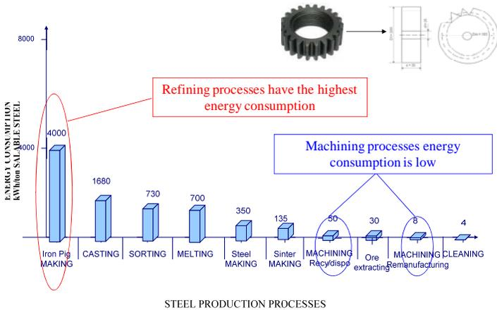
Figure 4: Steel Gear Energy Consumption [kWh/ton] [7]
