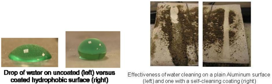
Figure 6: Water on untreated and self-cleaning aluminum [10]
